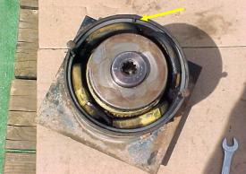
The splined socket is visible in the center of the armature. The finger key may be seen as a dark spot on the outer case of the motor, near the top of the photo.
